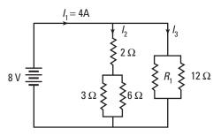
**34.** Find all of the equivalent resistance of the circuit and the current through each resistor.
