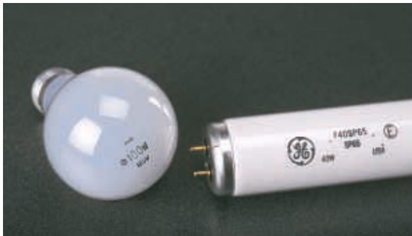
Figure 15.26 The power rating (sometimes called the “wattage”) of a light bulb tells you how fast it will convert electric energy into heat and light. For an incandescent bulb, only about 2 percent of the transformed energy is actually emitted as light; the rest is emitted as heat. A fluorescent bulb, on the other hand, converts about 9.5 percent of its energy into light, making it more than four times as efficient as an incandescent bulb.
